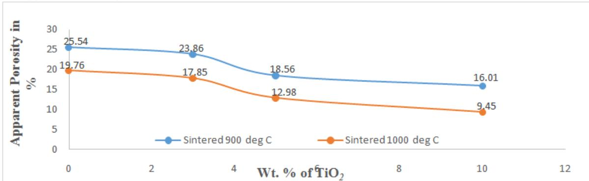
Figure 11: Apparent porosity for TiO<sub>2</sub>- TCP composites sintered at different temperatures
