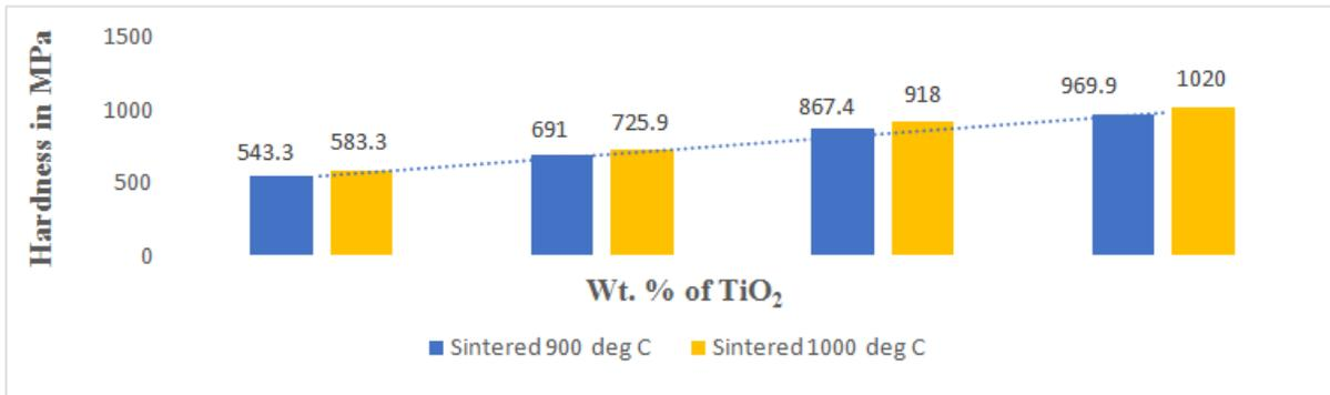
Figure12: Variation of hardness due to increment of TiO<sub>2</sub> into TCP matrix
