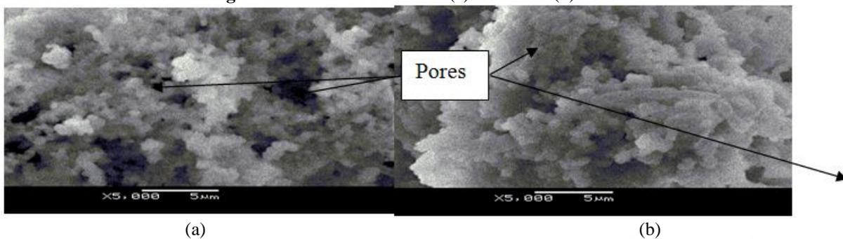
**Figure 6:**SEM image of 3Wt. % TiO<sub>2</sub>- TCP composite sintered at (a)900<sup>0</sup>C and (b) 1000<sup>0</sup>C
