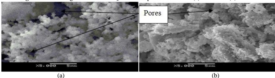
**Figure 7:** SEM image of 5 Wt. % TiO<sub>2</sub>- TCP composite sintered at (a)900<sup>0</sup>C and (b) 1000<sup>0</sup>C
