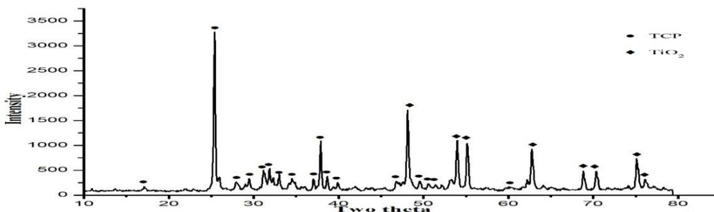
Figure 2: XRD pattern of  $\text{TiO}_2$ - TCP composite
