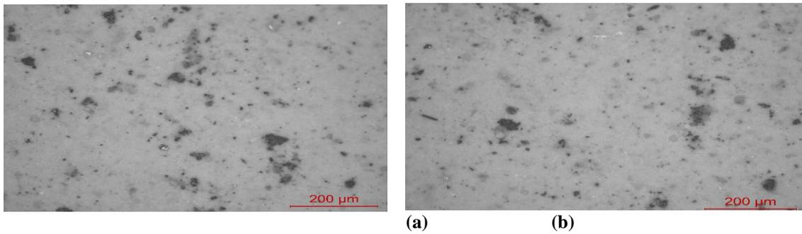
**Figure 4:**Microstructure by optical microscopy for (a) 3 Wt. % and (b) 5 Wt. %TiO<sub>2</sub>- TCP composite
