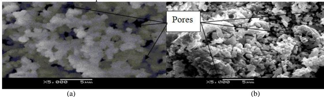
**Figure 5:** Pure TCP sintered at (a)900<sup>0</sup>C and (b) 1000<sup>0</sup>C
