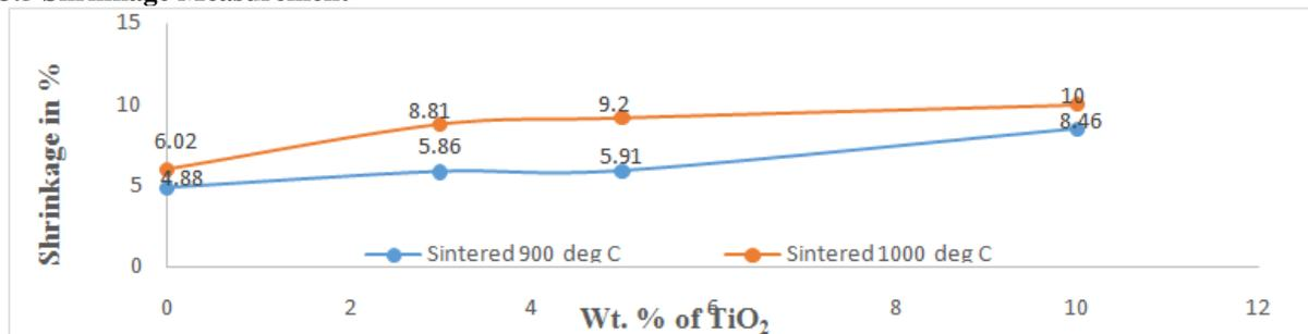
**Figure9:** Shrinkage for TiO<sub>2</sub>- TCP composites sintered at different temperatures
