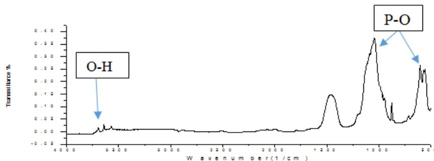
Figure 3: FTIR analysis for  $\beta$  TCP
