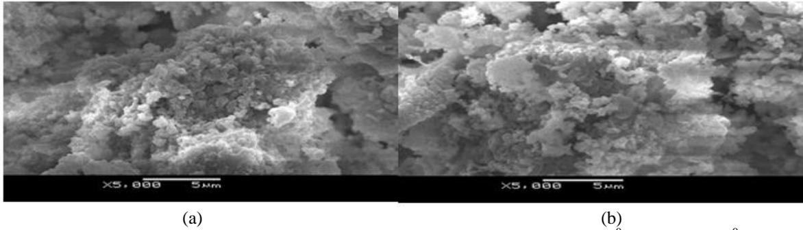
**Figure 8:** SEM image of 10 Wt. % TiO<sub>2</sub>- TCP Composite sintered at (a)900<sup>0</sup>C and (b) 1000<sup>0</sup>C
