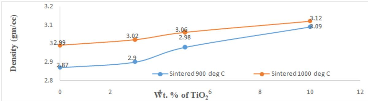
Figure 10: Density for TiO<sub>2</sub>- TCP composites sintered at different temperatures
